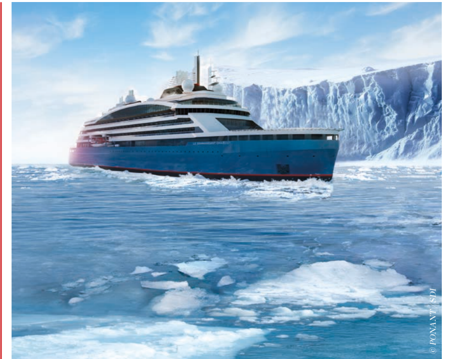
Bureau Veritas supporting innovation: PONANT's order for an ice breaking expedition class ship incorporates LNG as fuel for a hybrid electric propulsion system as well as an icebreaking hull.
