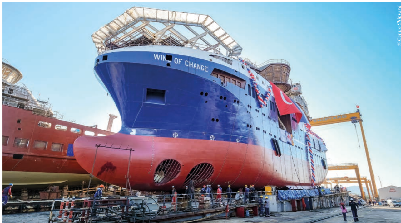
Hybrid and electric ships represented a growing trend in 2018, with particular bright spots in coastal shipping, passenger ships and offshore support vessels. In addition to classing Canada's first all-electric ferries, Bureau Veritas classed the Wind of Change, Louis Dreyfus Armateurs' award winning SOV. The ship is powered by an innovative hybrid-electric configuration - managed on a DC grid, to increase efficiency. This significantly reduces both fuel consumption and air emissions. As environmental regulations become stricter, our experts will continue to offer a range of services and notations for hybrid and electric vessels through 2019 and beyond.
