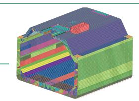
Our finite element software tool VeriSTAR Hull combines the well-known FEMAP processing tool and the proven NX and MSC Nastran solvers with in-house developed features for fast and efficient modelling and results assessment.
