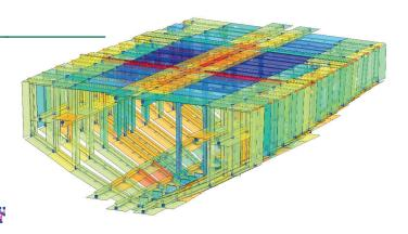
STEEL provides many types of profiles as well as beams with rigid ends, fully rigid beams, releases in all directions (global axis and local beam axis) and refined post-processing analysis in hole areas.
