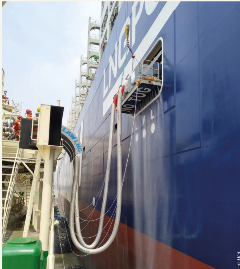
Teams at the shipyard test how to safely connect and disconnect the hose on the LNG BV.
