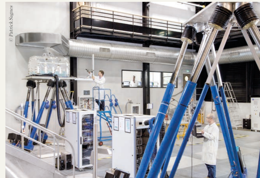
GTT's laboratory where tests are carried out on small tank models (hexapods) to calculate sloshing.
