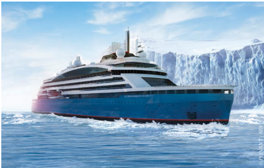
Bureau Veritas supporting innovation: PONANT's order for an ice breaking expedition class ship incorporates LNG as fuel for a hybrid electric propulsion system as well as an icebreaking hull.
